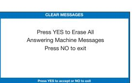
**Note:** The display screen indicates when Answering Machine memory is close to filling up, letting you clear messages before the memory is completely full. If Answering Machine memory becomes full, CapTel will not be able to record new messages until older messages are cleared from memory.
