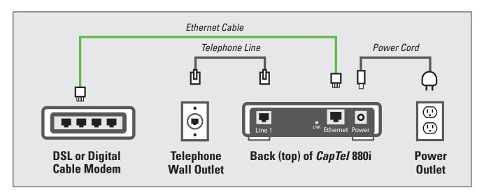
**Example 2:** If there is not an available Ethernet jack in your DSL or Cable Modem, you will need a router or switch that lets you connect more than one device to the Internet. Contact your Internet Service Provider to learn what router or switch will work with your modem. The router should support DHCP. Connect the router to your DSL/Cable Modem. Then connect the *CapTel* 880i to the router or switch using the Ethernet cable as shown below.
