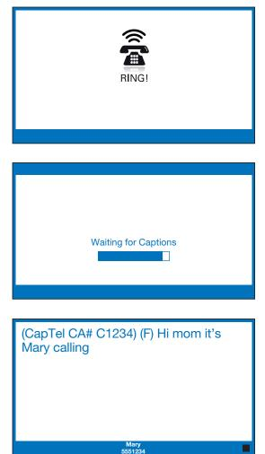
**TIP:** If you answer on an extension telephone and want to get captions, just pick up the CapTel handset. As long as the Line in Use feature is turned on, your CapTel phone will connect to the Captioning Service, and you will be able to view captions of the call on the CapTel display screen. For more options, see "Knowing when the Phone Line is Already in Use" on page 99.
