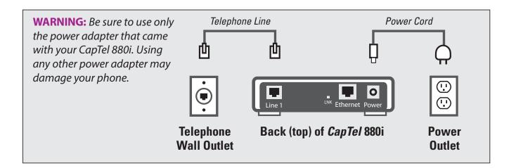
Once you plug in the power, your *CapTel* phone will automatically check that everything is connected and working properly. You can follow along on the *CapTel* display screen, which will tell you what is happening during the setup process.
